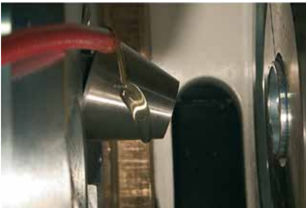
Before beginning the flaring operation check that the surface of the flaring cone has been thoroughly oiled or treated with Gleitmo 830 (Fuchs Lubritech) lubricating paste for cold forming.
