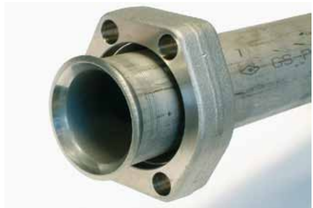
The flared pipe is cleaned with a cloth before visually checking quality.
