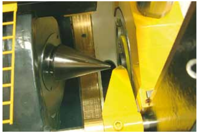
The pipe end is inserted into the dies with the correct flaring dimensions.
