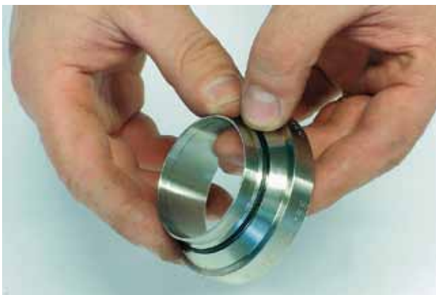
Lubricate the O-ring with Gleitmo 750 or equivalent lubricant. Place O-ring carefully into its groove. Examine all sealing surfaces to detect possible rust or mechanical damages.
