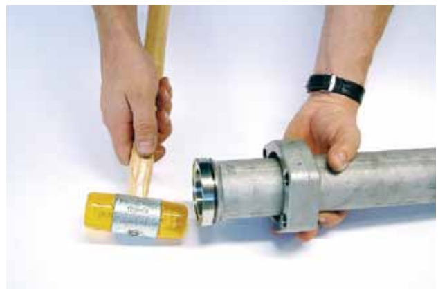
Fit the insert cone into the tube flare. If needed, tap gently with plastic or hide mallet.
