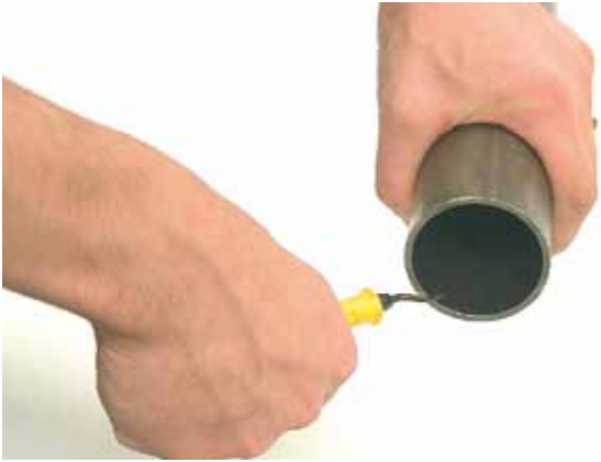
The pipe is first deburred inside and out.
