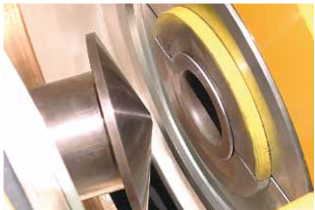
The pipe is flared in two stages, first 37° and then 90°.
