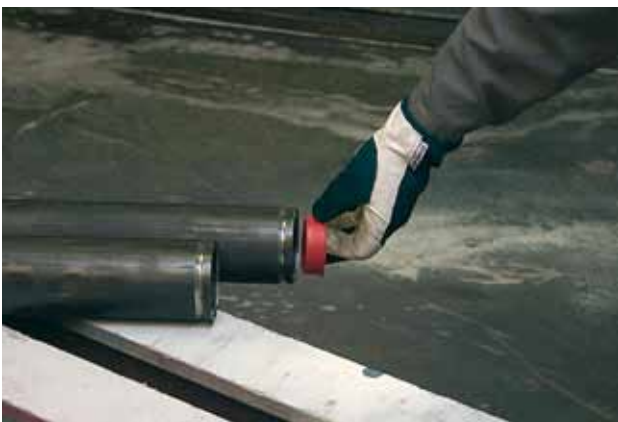
Prior to shipping the pipe end is carefully plugged.
