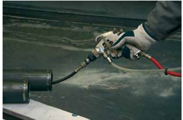
Piping modules are protected with oil in order to prevent corrosion during transportation and storing.
