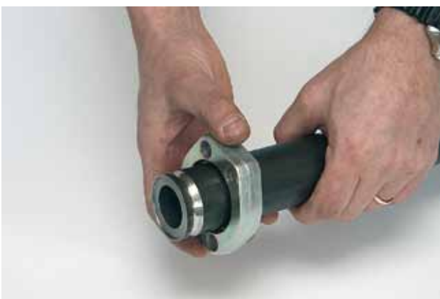
Install the flanges with the retain ring groove facing towards the end of the pipe. Please use the original GS-Hydro flanges to ensure a leak-free connection.
