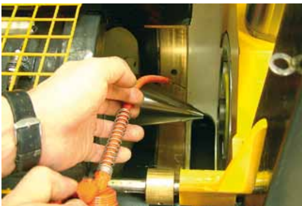
The cone and inside the pipe is lubricated.
