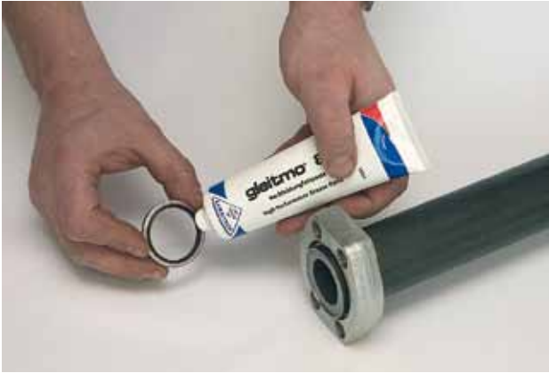
Lubricate the bonded seal with Gleitmo 805 -paste or equivalent. Control that pipe ends fit together and are aligned for sealing.
