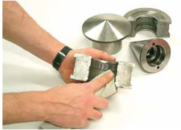
The flaring cone and dye is cleaned before beginning the flaring.
